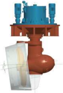
可倾斜的集成式舵桨 Tilttable Integrated Azimuth Thruster
