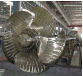
可调桨车间装配调试 CPP assembly& commissioning at workshop
