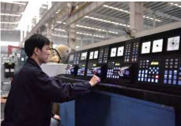
可调桨车间装配调试 CPP assembly& commissioning at workshop
